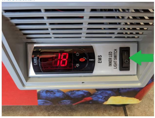
This switch turns the internal **light** on/off. It does **NOT** turn the machine on/off!
