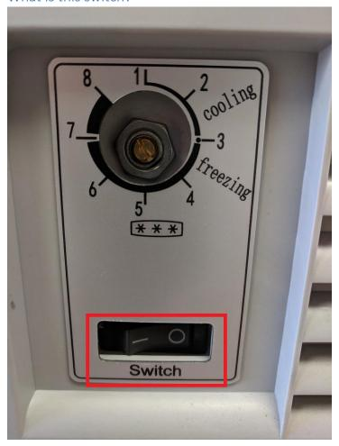
This switch turns the internal **light** on/off. It does **NOT** turn the machine on/off!
